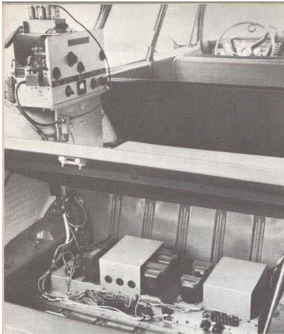
INSTALLATIONS OF POWER SUPPLIES and linear amplifiers in W8DLD's (left) and W8WFH's (right) station wagons. Storage compartments under cargo decks are handy locations for high voltage power supplies, while r.f. equipment is fastened to shelves atop rear wheel housings.
